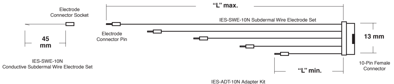
IES-SWE-10N Subdermal Wire Electrode Set & IES-ADT-10N Adapter Kit
